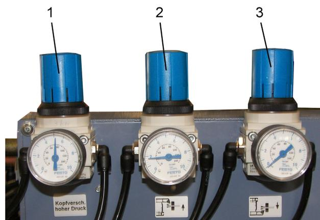
Figure 3.2-3: Pressure controller at each welding head (depending on the machine equipment)
