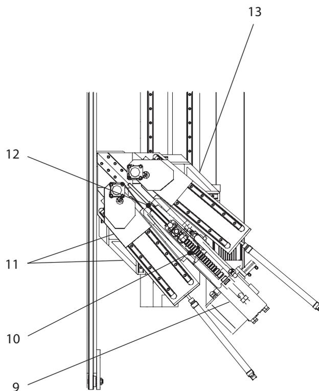
Figure 7.4-3: Lubricating points at welding heads
