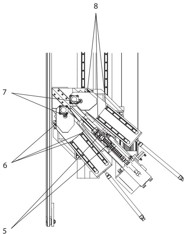
Figure 7.4-2: Lubricating points at profile clamping and heat plate
