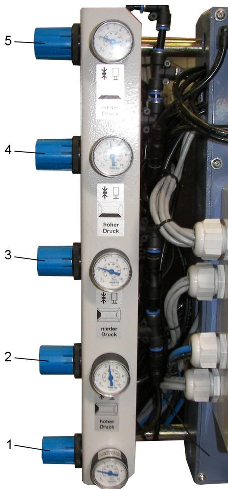
Figure 3.2-2: Pressure controller at each welding head
