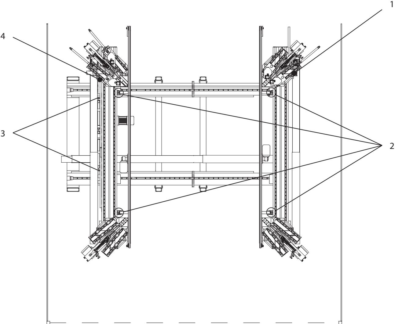
Figure 7.4-1: Lubrication plan (representation of the machine without control panel)
