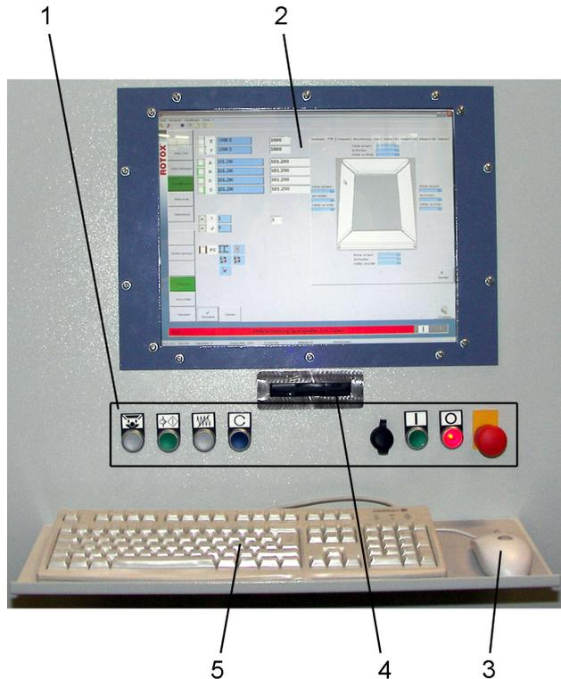
Figure 3.2-1: Operating elements at the control box (machine with fixed side on the left)
