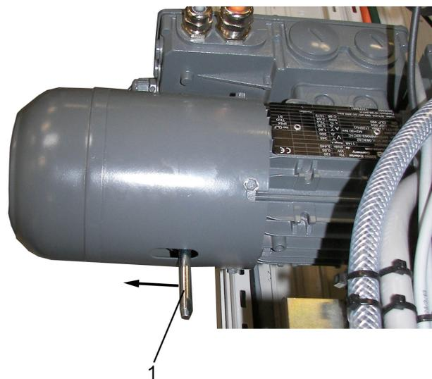
Figure 3.2-4: Brake of the axis motors
